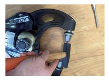
Then tap the new tip carefully into the crusher arm's receptacle using a small hammer until it locks in completely.
