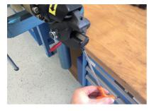
The relevant Allen screw must be removed completely to replace the triangular cutting blades. The entire cutting blade can then be pulled forwards out of the guide. The blade also has two slots for this, which can be pulled using a pliers.
