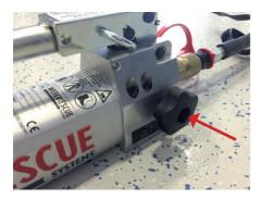
The hand wheel to control the oil flow is located on the right side of the hand pump. The wheel must be turned in a clockwise direction until it reaches the stop in order to establish pressure in the cylinder.
