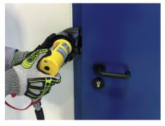
Option 1 is to break open the lock. To do this, the door opening cylinder is pushed in or hammered in with the claw and foot between the doors and the door frame (about one hand width above or below the lock).
