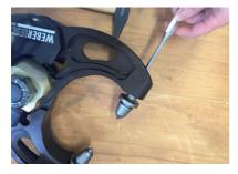
If the tips on the concrete crusher are worn, they can be replaced with new tips quickly and easily.
