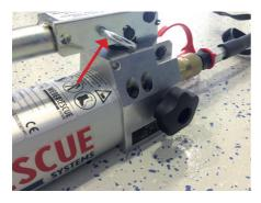
In addition, the hand pump has a locking hook for the pump lever. This hook can be used to connect the lever to the pump housing and therefore to use it as a carrying handle.
