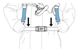
Pull down on the lower shoulder strap (6) ends until the apparatus fits comfortably.
