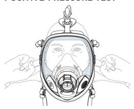
With the cylinder valve open, insert a finger under face-seal and check for a steady outward flow of air. Remove finger and allow mask to re-seal.
