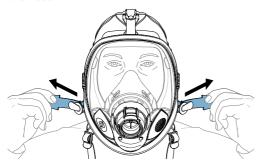
Tighten harness side straps. DO NOT OVER-TIGHTEN.
