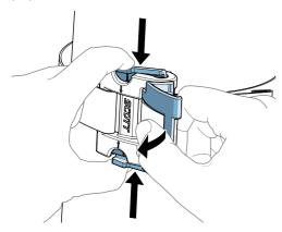
Simultaneously depress the two cylinder buckle buttons and pull the cylinder buckle (22) to release from the cylinder. Loosen cylinder band (18) and remove the cylinder by sliding it in either direction.
