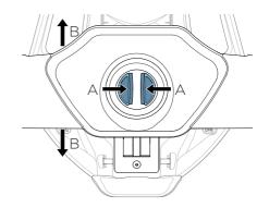
Using the fingers and thumb, squeeze together the two halves of the release catch (A).
