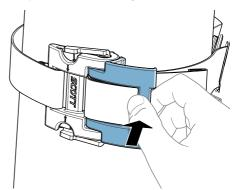
Push the cylinder buckle (22) to the closed position.
