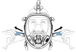
Adjust the facemask top strap so that the mask is at the correct level with the face and the head-harness pad is in the centre of the back of the head. Tighten harness straps in sequence: **Bottom, Middle, Top.** DO NOT OVER-TIGHTEN.
