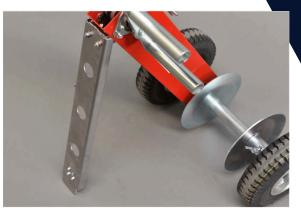
ROLLY III SUPPORT FOOT for fast and secure parking of the Rolly at the scene, so the Rolly can be used quickly for coiling center folded hoses and is protected from damage. The support food of galvanized steel is held magnetically to the body of the Rolly and can be easily expanded by foot.
