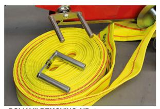
ROLLY III REMOVING AID for center folded (dutch/double stile) coiled hoses The magnetically adhering sleeve on the winding fork ensures effortless shedding of firm and center folded hoses. After the hose is coiled the removing aid can be dropped of with the hose by lateral tilting of the Rolly. The removing aid can be easily taken away from the hose coil and be placed back on the winding bolts.
