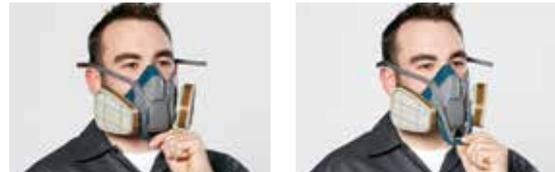
**TO CLOSE QUICK LATCH:** Grasp the face piece with your thumb on the bottom of the face piece and your first two fingers on top of the latch. Place the face piece over your nose and mouth while pushing down on the latch.
