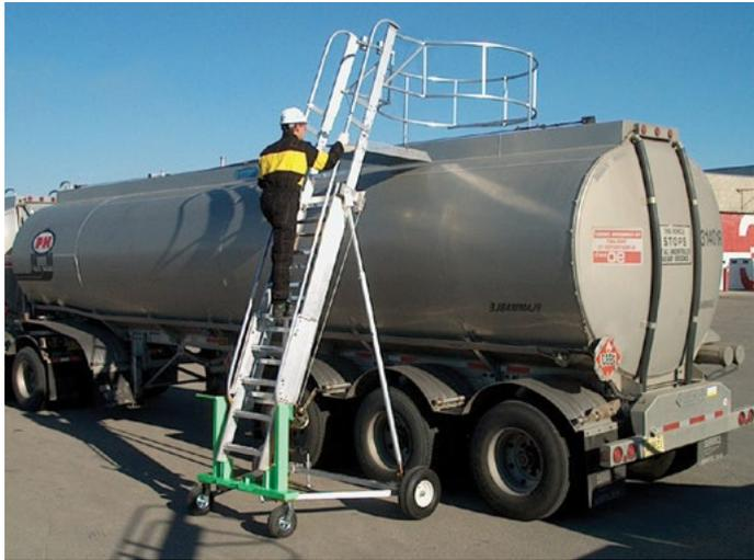
**Portable tanker access ladder system - work positioning.**
